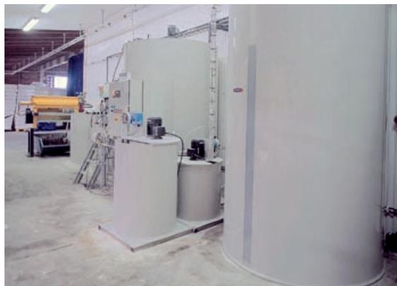
Neutralisation of rinse water after pickling with Avesta-BML Neutralising Facility.
